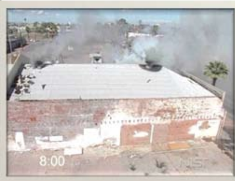
Eight minutes after ignition, the two glass doors at the front of the warehouse were broken to simulate forcible entry by firefighters. The palm tree is directly across from the six-by-10-foot front glass door.
