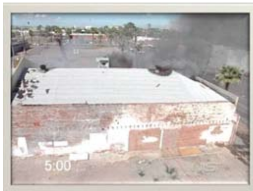
Five minutes after ignition, exterior conditions look similar to the three photos. Notice that the smoke that was venting along the top of the wall at four minutes has vanished.
