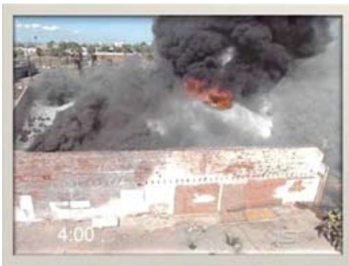
Four minutes after ignition, with abundant heat, fuel and oxygen, the fire is feasting as flashover temperature is reached. The average temperature throughout the warehouse three
